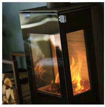
Our Advanced Glass Concept® effectively minimises soot build-up on wood stove glass and ensures that you can always enjoy a beautiful view of the flames through clean panes. Soot build-up is avoided by getting to operational temperatures quickly and by ensuring high temperatures in the combustion chamber. We ensure this process by using **coated glass and two-layered glass** that reflect the radiant heat. Read more about our Advanced Glass Concept® on page 86.
