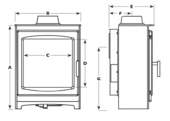
A 604mm C 349mm E 321mm G 452mm B 466mm D 344mm F 161mm
