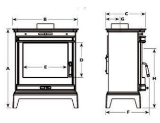
A 637mm C 326mm E 360mm G 113mm B 532mm D 275mm F 352mm H 506mm
