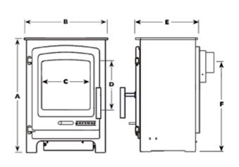
A 568mm C 260mm E 305mm B 413mm D 237mm F 450mm
