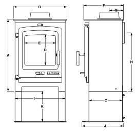
A 588mm C 260mm E 247mm G I 12mm I 390mm K 250mm B 414mm D 249mm F 295mm H 451mm J 330mm
