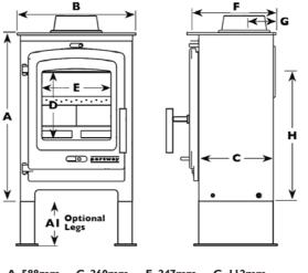
A 588mm C 260mm E 247mm G II2mm B 414mm D 249mm F 295mm H 451mm AI 150/300mm
