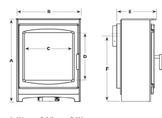
A 604mm C 349mm E 290mm B 466mm D 344mm F 478mm
