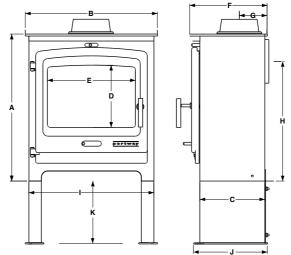
A 588mm C 260mm E 350mm G II2mm I 500mm B 524mm D 254mm F 310mm H 451mm J 310mm K 150/300mm High/Low Legs
