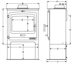
A 588mm C 260mm E 350mm G II2mm I 500mm K 250mm B 524mm D 254mm F 310mm H 451mm J 330mm
