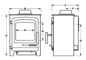
A 573mm C 260mm E 346mm G 463mm **B 413mm D 237mm F 163mm** (138mm using optional flue casting collar)
